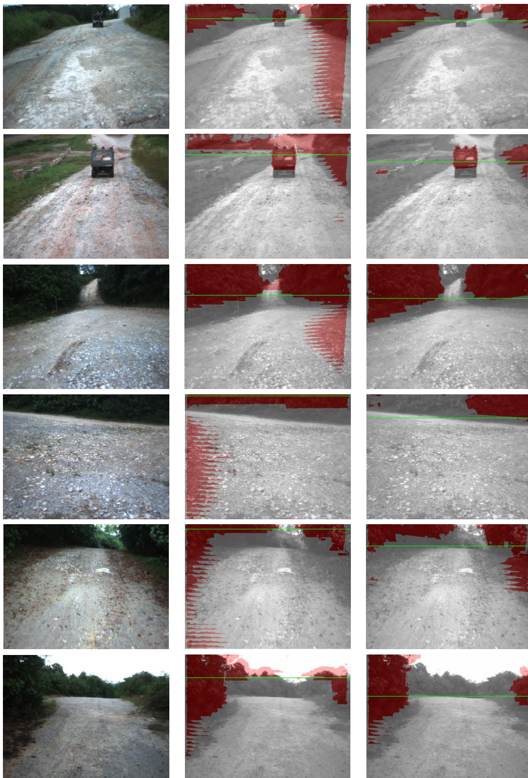
FIGURE 6.22: Performance comparison I: left - reference image, center - planar ground approximation, right - proposed algorithm.
