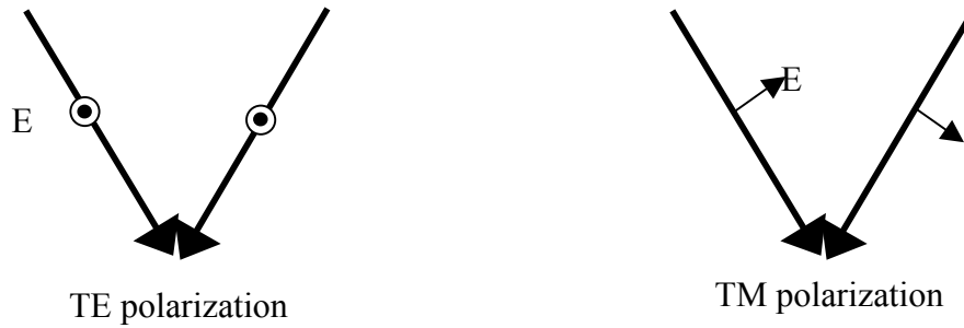
Fig. 2.36 TE and TM polarization of electric field
