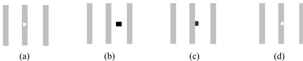
Fig 2.9 Types of defects classified by location: (a) pinhole, (b) post, (c) clear extension, (d) dark extension
