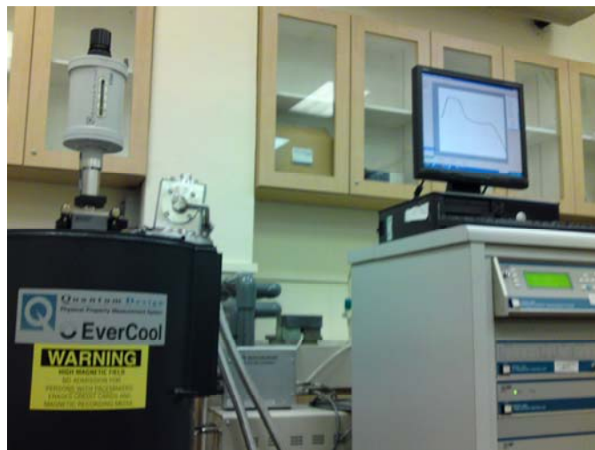
Fig. 2. 1: Photograph of the Vibrating Sample Magnetometer (VSM) module attached to Physical Property Measurement System (PPMS)
