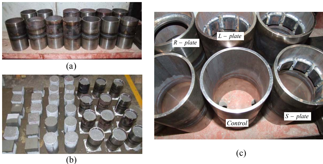
Figure 4.35 Small scale column stubs: (a) external view of un-grouted specimens; (b) infill grouted specimens with grout samples; (c) internal view of un-grouted specimens
