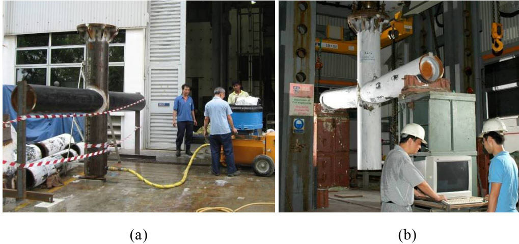
Figure 6.1 Research for grouted tubular joints conducted in NUS: (a) grouting the cross joint; (b) in-plane bending test
