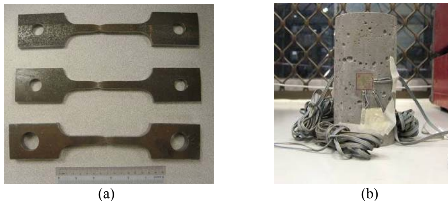
Figure 4.2 Material test samples: (a) failed steel coupons; (b) grout cylinder ready for test
