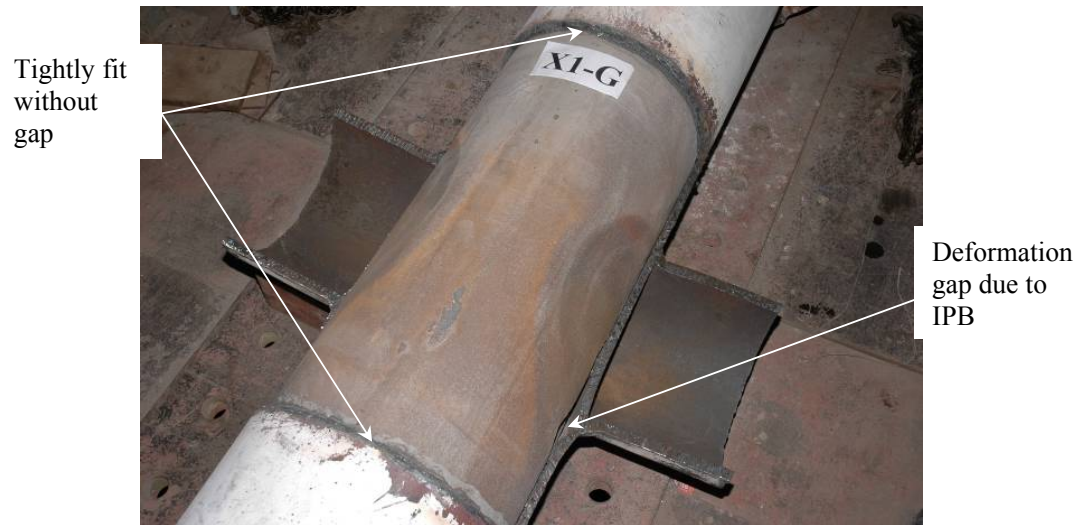
Figure 6.6 Open-up of the grouted specimen after test
