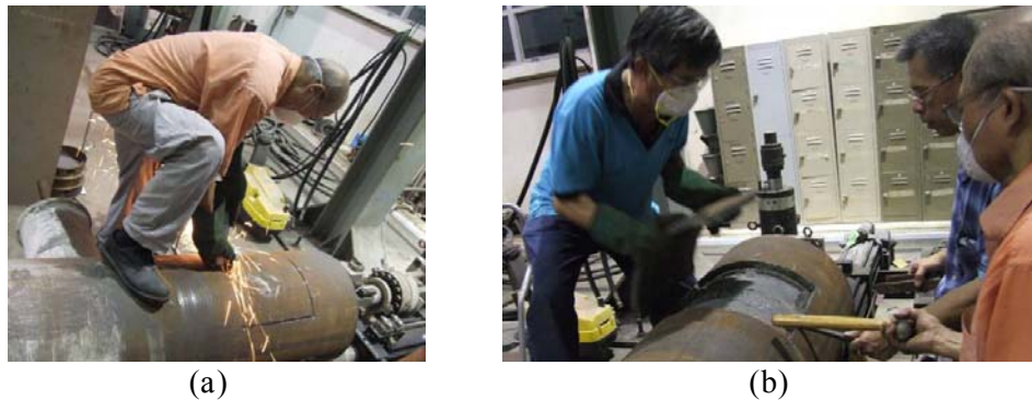
Figure 4.6 Open the tested G1: (a) manual saw cutting; (b) opening up
