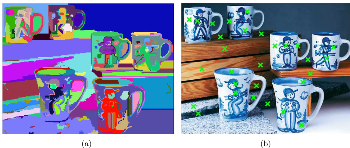
Figure 8.4: The possible fixation locations in the image are shown by green "X"s in (a). These are the centers of the regions from the color based segmentation of that image in (b)
