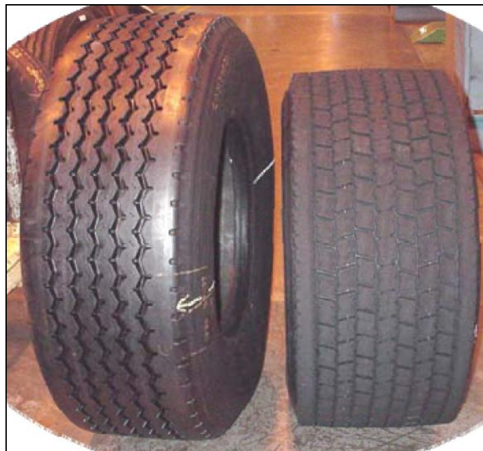
Figure 4.2 Wide-Base Truck Tires (425/65R22.5 and 455/55R22.5)
