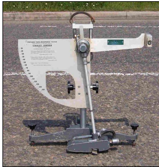
Figure 2.10 British Pendulum Tester (BPT)
