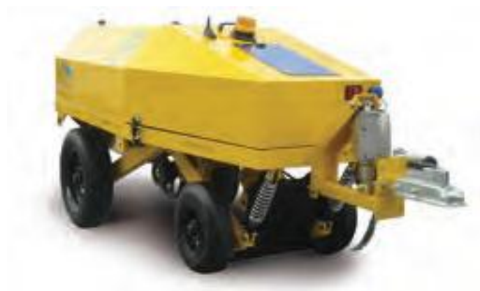
Figure 2.11 Dynamic Friction Tester (DFT)
