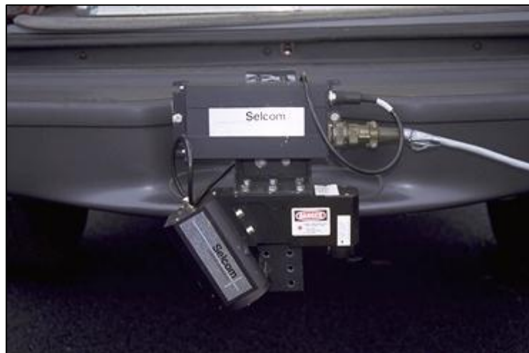
Figure 2.15 Prototype ROSAN devices
