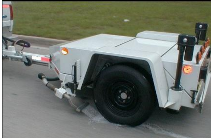
Figure 2.12 Locked-wheel skid resistance testers
