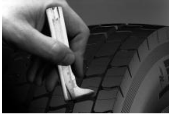
Figure 5.4 Schematic of Tread Depths Measurement
