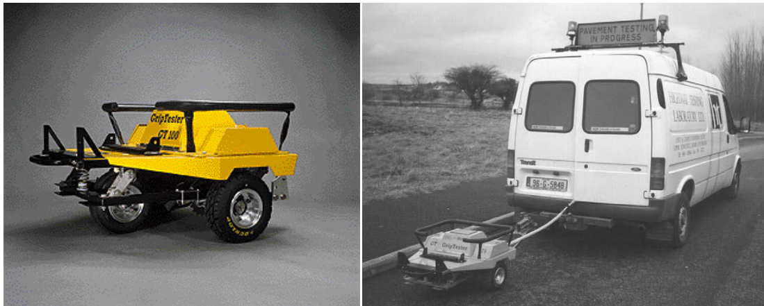
Figure 2.14 Griptester for skid resistance testing
