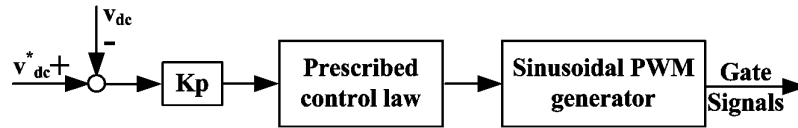
Fig.2.2 Schematic diagram for indirect current control or phase and amplitude control
