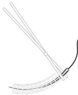
Figure 4.2: Sliding an arc along a circular path is one of the dexterity primitives we use to learn maneuvering a needle in microsurgery
