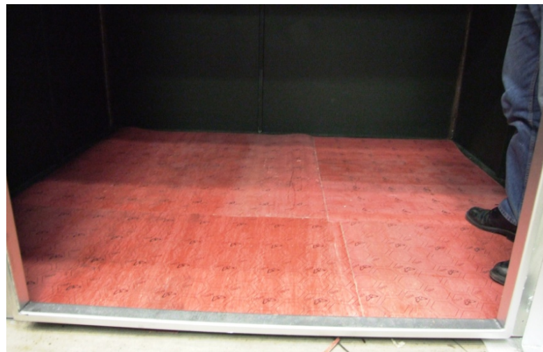
Figure 9.19 the thermal insulation beneath the chamber's base plate
