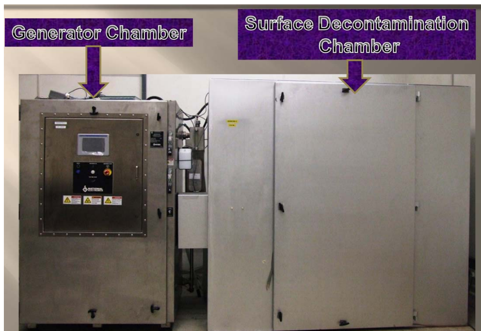
Figure 9.21 The large chamber connected to the generator's cabinet
