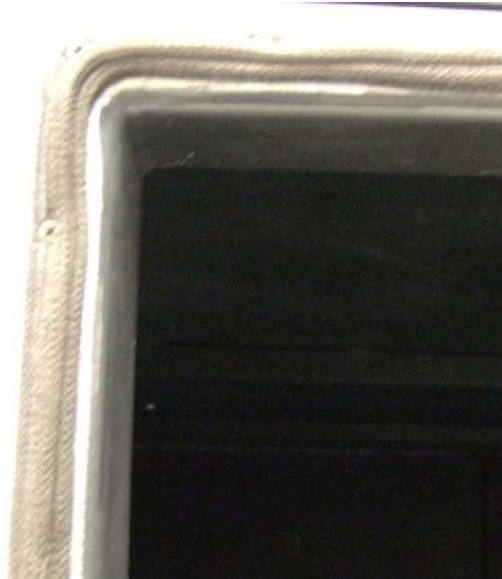
Figure 9.20 RF Gasket of the chamber's door
