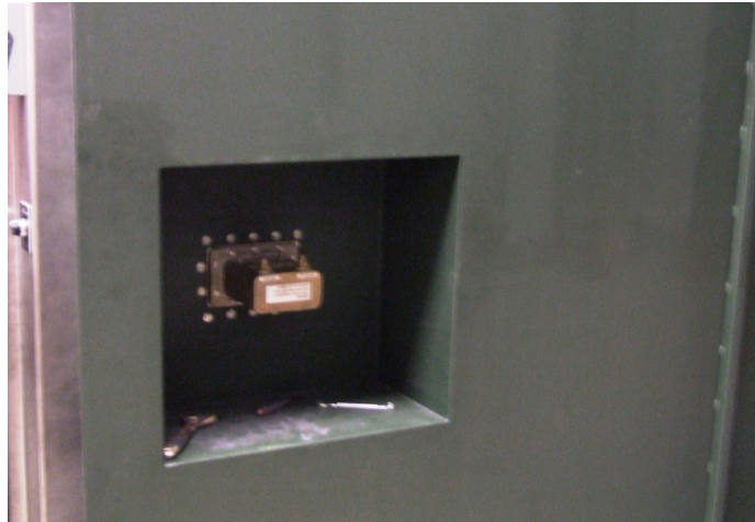
Figure 9.18 Small tunnel to connect the chamber to the generator's cabinet
