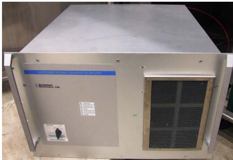
Figure 9.3 Switch mode power supply
