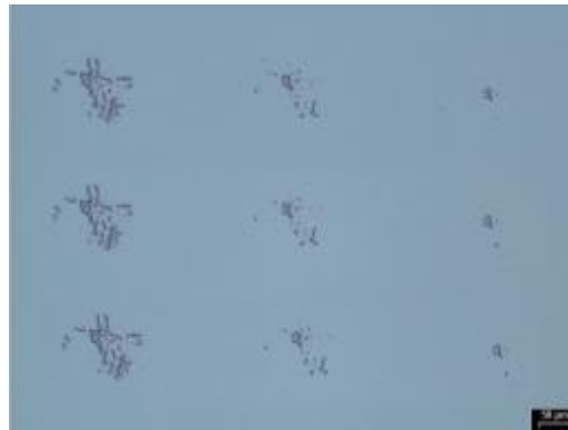
Figure 4.49 OM images of 100 nm \text{Ag}_5\text{In}_5\text{Sb}_{30}\text{Te}_{60} films at amorphous background after single femtosecond pulse irradiation. Pulse energy from left to right: 16 \mu\text{J} , 14 \mu\text{J} and 12 \mu\text{J} .
