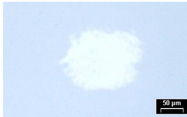
Figure 6.14 OM image of 100 nm amorphous superlattice-like phase change media after irradiation by single femtosecond at the energy of 14 \mu\text{J} .
