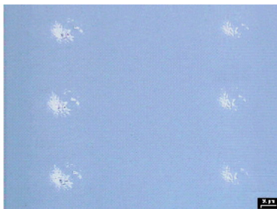
Figure 4.44 OM images of 100 nm \text{Ge}_1\text{Sb}_2\text{Te}_4 films at amorphous background after single femtosecond pulse irradiation. Pulse energy from left to right: 21 \mu\text{J} and 18 \mu\text{J} .
