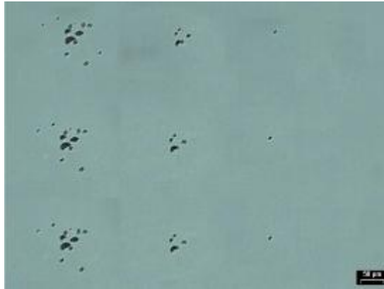
Figure 4.36 OM images of 60 nm \text{Ge}_2\text{Sb}_2\text{Te}_5 films at amorphous background after single femtosecond pulse irradiation. Pulse energy from left to right: 13 \mu\text{J} , 12 \mu\text{J} , 10 \mu\text{J} , and 9 \mu\text{J} .
