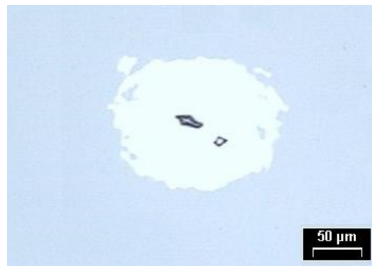
Figure 5.5 OM image of 100 nm amorphous \text{Ge}_2\text{Sb}_2\text{Te}_5 films after exposure to single femtosecond pulse at the energy of 15 \mu\text{J} .
