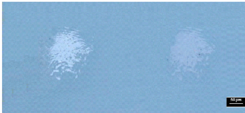
Figure 4.30 OM images of 100 nm Ge 2 Sb 2 Te 5 films at amorphous background after (left) single pulse irradiation at the energy of 36 μJ and (right) two pulses irradiation. First pulse energy: 36 μJ; Second pulse energy: 21 μJ.
