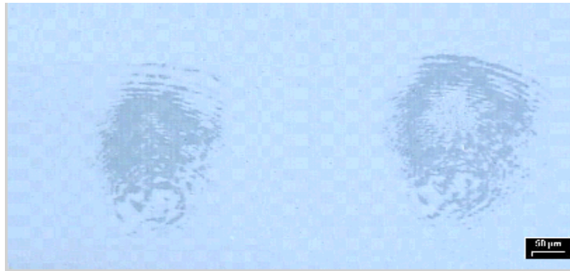
Figure 4.29 OM images of 100 nm Ge 2 Sb 2 Te 5 films at crystalline background after (left) single pulse irradiation at the energy of 24 μJ and (right) two pulses irradiation. First pulse energy: 24 μJ; Second pulse energy: 30 μJ.
