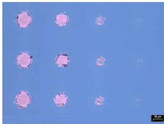
Figure 6.7 OM image of 20 nm superlattice-like phase change media at amorphous background after single femtosecond pulse irradiation. Pulse energy from left to right: 12 μJ, 10 μJ, 8 μJ, and 6 μJ.
