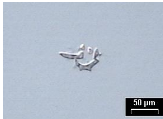
Figure 5.4 OM image of 100 nm amorphous \text{Ag}_5\text{In}_5\text{Sb}_{30}\text{Te}_{60} films after exposure to single femtosecond pulse at the energy of 15 \mu\text{J} .
