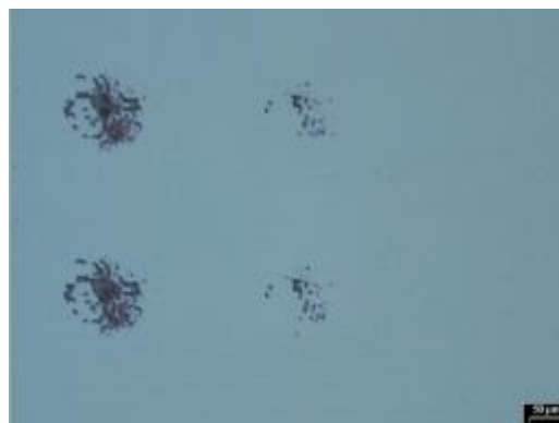
Figure 4.47 OM images of 20 nm \text{Ag}_5\text{In}_5\text{Sb}_{30}\text{Te}_{60} films at amorphous background after single femtosecond pulse irradiation. Pulse energy from left to right: 12 \mu\text{J} , 10 \mu\text{J} and 8 \mu\text{J} .
