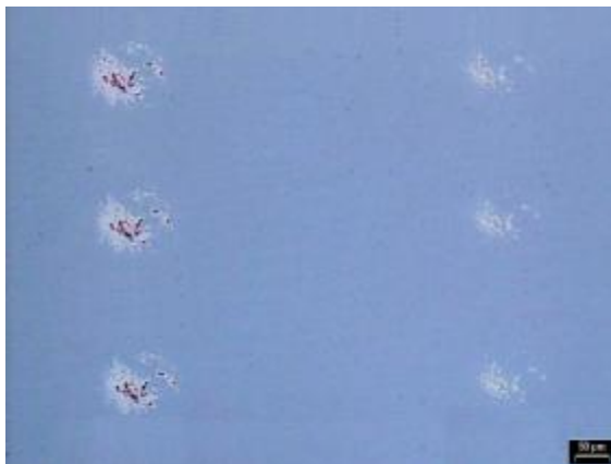
Figure 4.25 OM images of 100 nm \text{Ge}_2\text{Sb}_2\text{Te}_5 films at amorphous background after single femtosecond pulse irradiation. Pulse energy from left to right: 21 \mu\text{J} and 18 \mu\text{J} .
