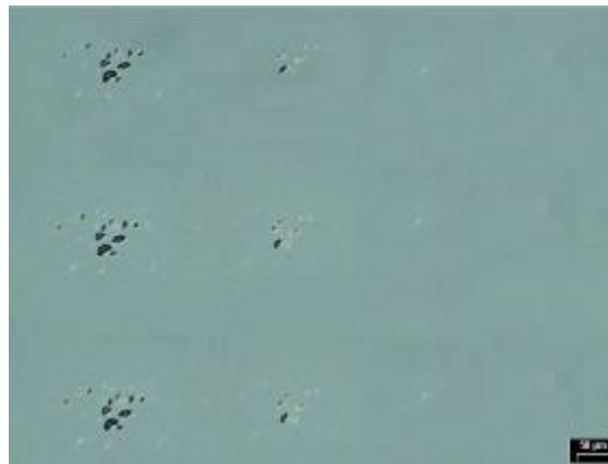
Figure 4.40 OM images of 65 nm \text{Ge}_2\text{Sb}_2\text{Te}_5 films at amorphous background after single femtosecond pulse irradiation. Pulse energy from left to right: 13 \mu\text{J} , 12 \mu\text{J} , 10 \mu\text{J} , and 9 \mu\text{J} .
