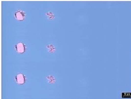
Figure 4.42 OM image of 20 nm \text{Ge}_1\text{Sb}_2\text{Te}_4 films at amorphous background after single femtosecond pulse irradiation. Pulse energy from left to right: 16 \mu\text{J} , 14 \mu\text{J} , 12 \mu\text{J} and 10 \mu\text{J} .
