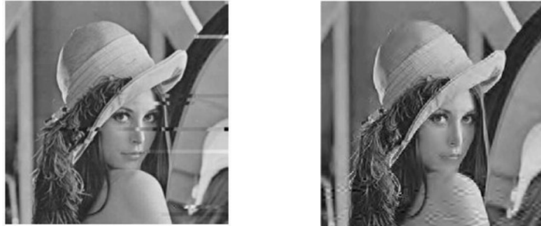
Figure 4-1 Corrupted images by channel BER 3 \times 10^{-4} (left: encoded by DCT 8 \times 8 block; right: Daubechies 9/7 DWT, block size 64 \times 64 )
