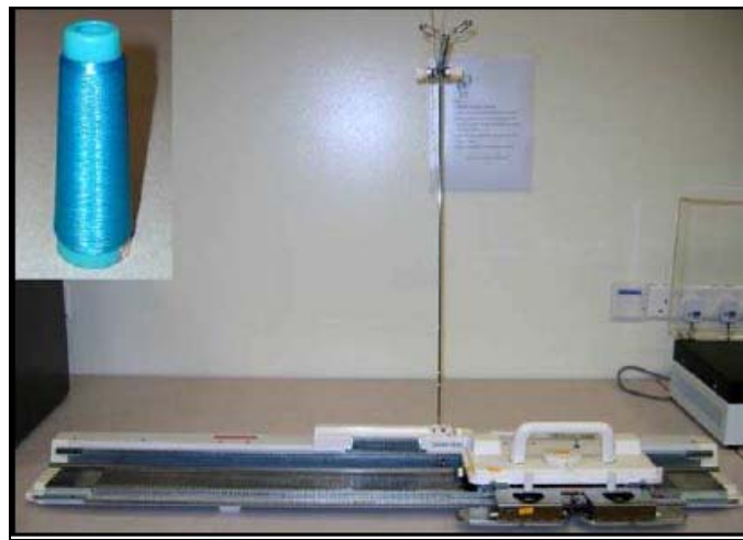
Figure 5.2: Knitting machine used to fabricate knitted scaffolds from PLGA fibres; Inset: Bundle of PLGA yarn.
