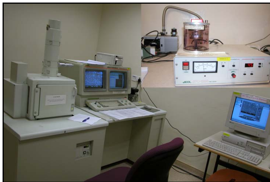
Figure 5.8: SEM, JEOL JSM-5800LV scanning electron microscope, Inset: JFC-1200 Fine coater, JEOL
