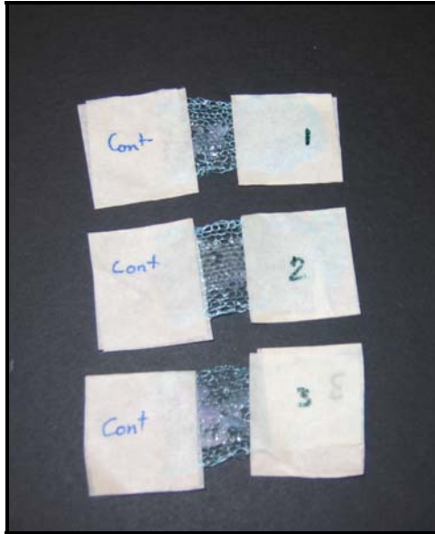
Figure 5.15: Samples for mechanical test with masking tape
