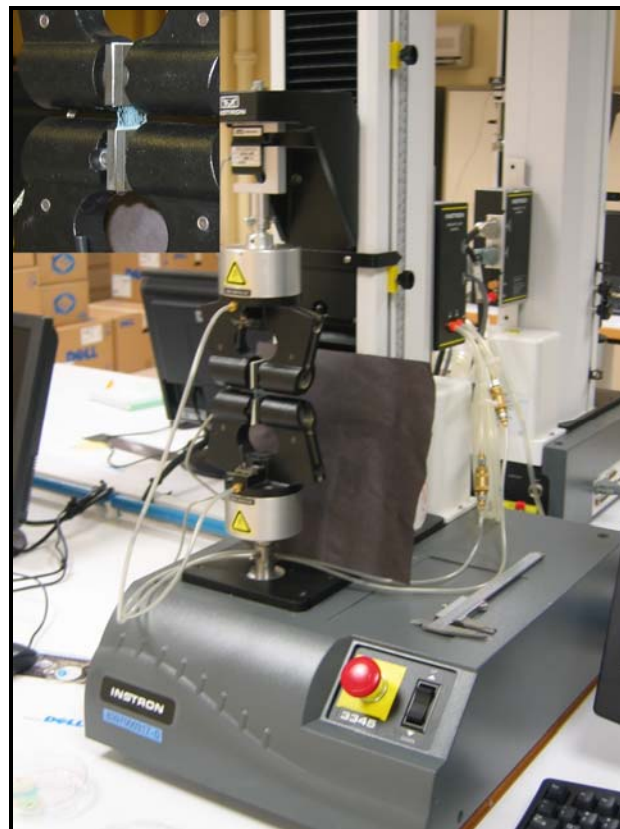
Figure 5.14: Universal testing machine (UTM) (Instron ® 3345 Tester) Inset: Close up view of sample on clamp
