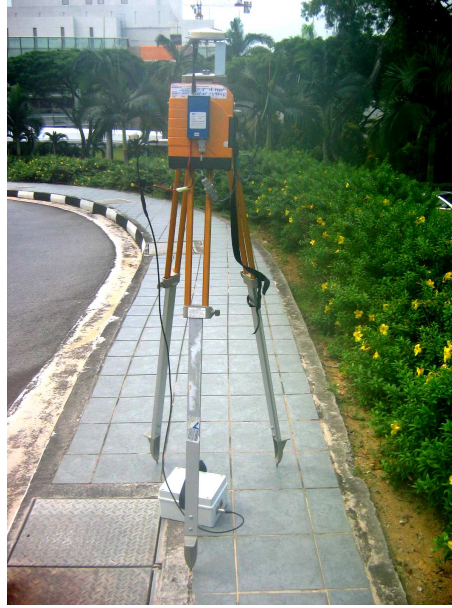
Figure 3.32: Base Unit for RTK GPS.
