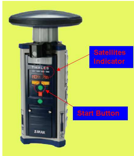
Figure A.6: Z-Max Surveying System
