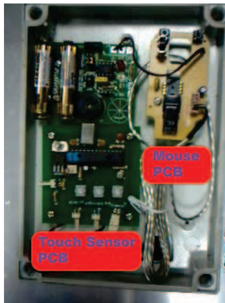
Figure 3.13: Touch Sensor and USB Mouse PCB in one PCB Housing
