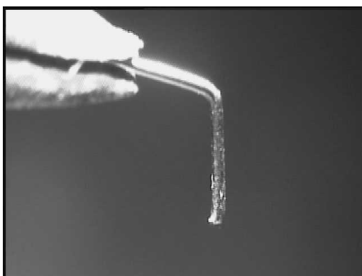
A) Tungsten rod bent for electrolyte etching.
