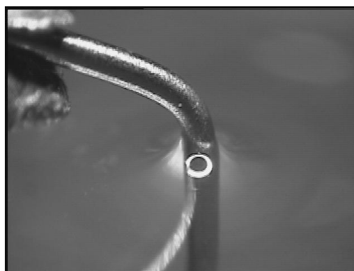
B) Etch tungsten rod to a certain diameter.
