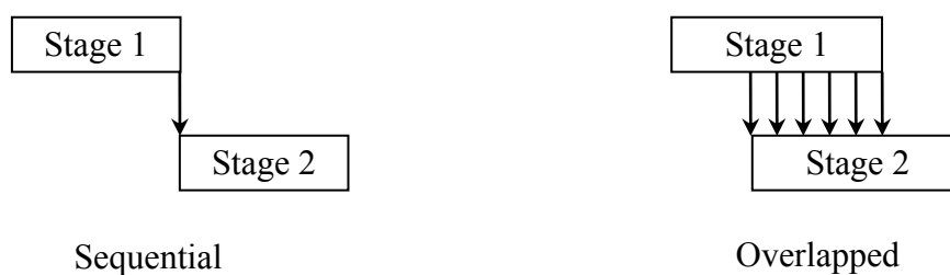
Figure 1.1 Sequential and overlapped NPD processes
