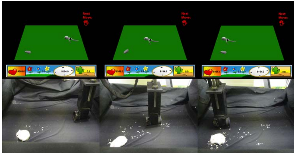
Figure 3.24: Human avatar position causes correspondingly the change of position of the mechanical arm. Note again the virtual hamster position corresponds to the physical live hamster position
