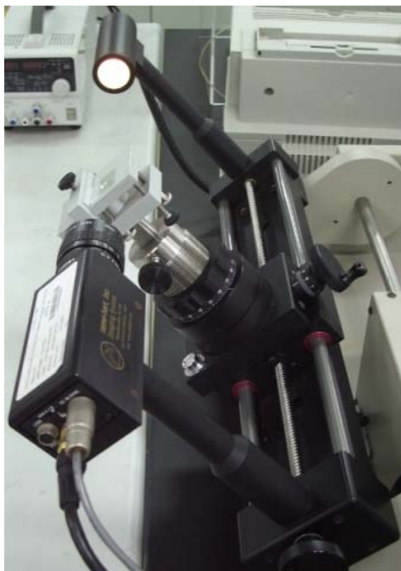
Figure 3.8: Entire goniometer set-up is tilted with the sample, in order to capture images for the measurement of advancing and receding contact angles.
