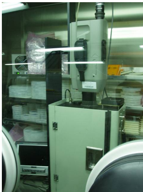
Figure 4.23: OLED current-voltage-luminance ( I-V-L ) measurement instrument.
