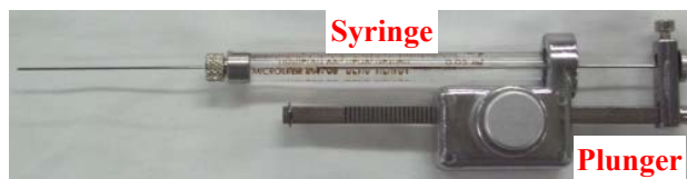
Figure 3.5: Syringe and plunger system used to deposit the one micro-liter droplet onto the sample. The needle tip is suggested to be flat-ended and not a tapered sharp point.
