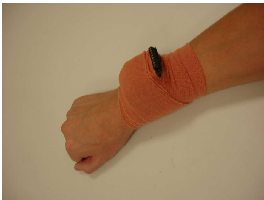
Figure 4.6: Illustrations of the activity detection testbed. Wrist-worn accelerometer was used for hand movement detection
