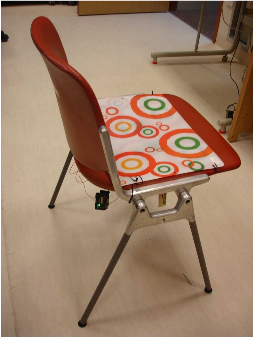
Figure 4.8: Illustrations of the activity detection testbed. Pressure sensors installed in the pad on the chair were used to detect if a person is sitting
