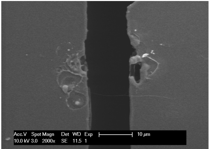
Figure 4.1 SEM image of a nanowire grown on a Si TEM die (3x3 mm 2 ).
