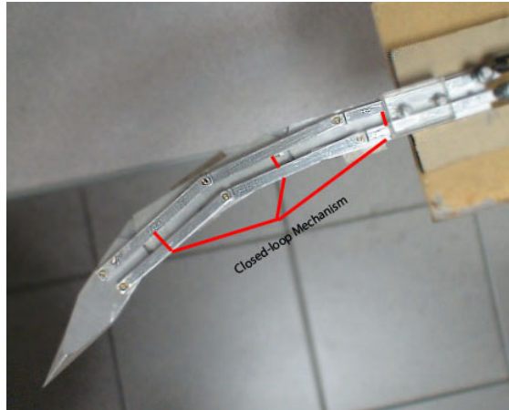
(a) Closed-loop mechanism consists of three parallel bars
