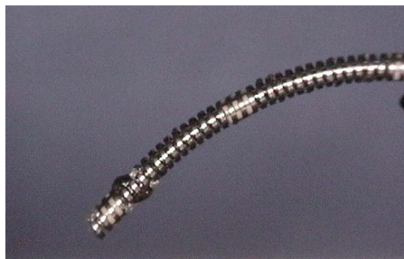
Figure 3.4: Small diameter active catheter using shape memory alloy coils [93]
