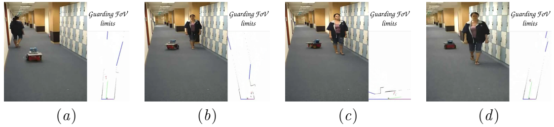
Figure 3.30. When the target doubles back, the tracker has to guard against its fov limits and makes a turn as well. (Video-id: Vantage-FoV)
