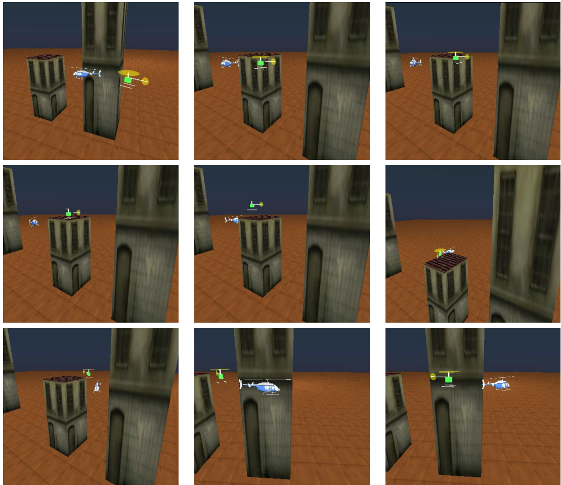
Figure 5.16. A set of snapshots showing the tracker's climbing behavior. The green tracker helicopter tracks the blue target helicopter using on board 3-D range sensor. We can see the tracker climb the shorter building and keep track of the target which is making a turn around the building. Again, when the target turns around the taller building, the tracker starts following it. (Video-id: Vantage3D-climb)
