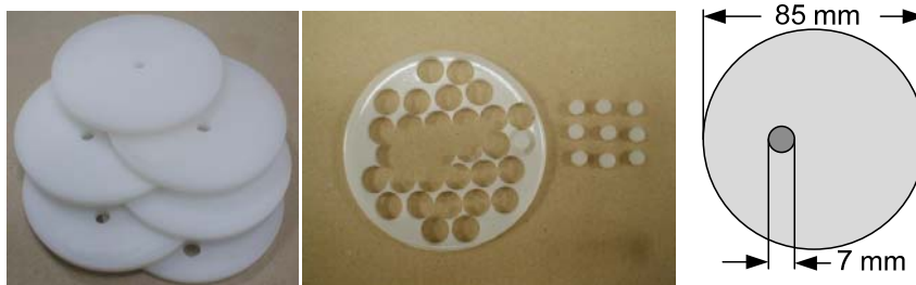
Fig. 5-1 (Left) Phantom discs with holes at different positions. (Center) Tumor-like phantom. (Right) Dimensions of the optical phantom.
