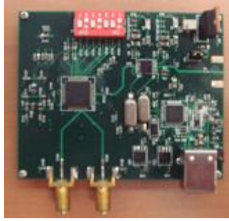
Fig. 4-9 PRBS generator using transceiver.
