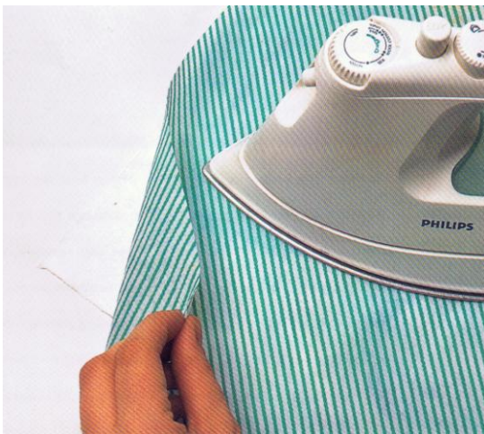
FIGURE 7-20 DRY PRESSING USING AN IRON
