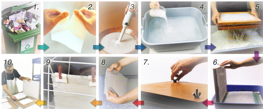
FIGURE 7-21 THE SYSTEM FLOW CHART OF PAPER RECYCLING THROUGH PAPERMAKING BY HAND
