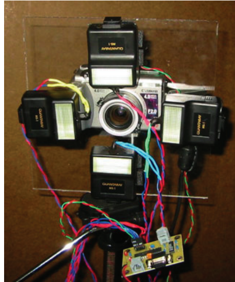
Figure 2.4: A prototype of multi-flash camera invented by Raskar et al. in [2004c]
