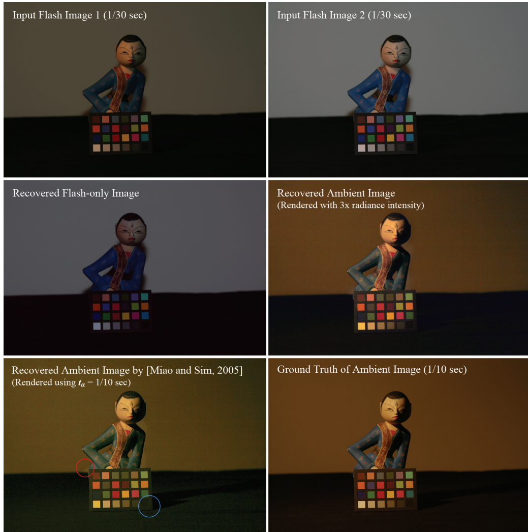
Figure 5.9: Our method can faithfully recover the ambient image. In overall, our result exhibits more accurate color than Miao and Sim’s. In details, our ambient recovery presents higher visual quality w.r.t. shadow separation (note the region in the red circle) and noise suppression (note the region in the blue circle).
