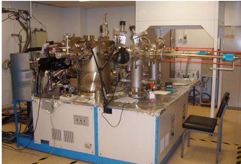
Figure 2-1: MBE system at the Centre for Optoelectronics.
