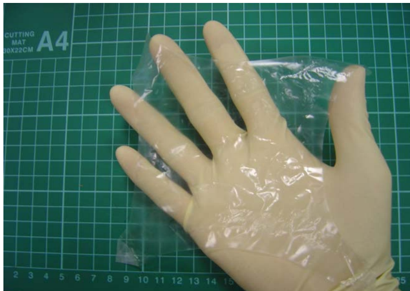
Figure 2-5 Ultra-thin PCL membrane by 2-roll-heated-mill methods. The membrane is transparent, mechanical strong and less than 10 \mu\text{m} in thickness.
