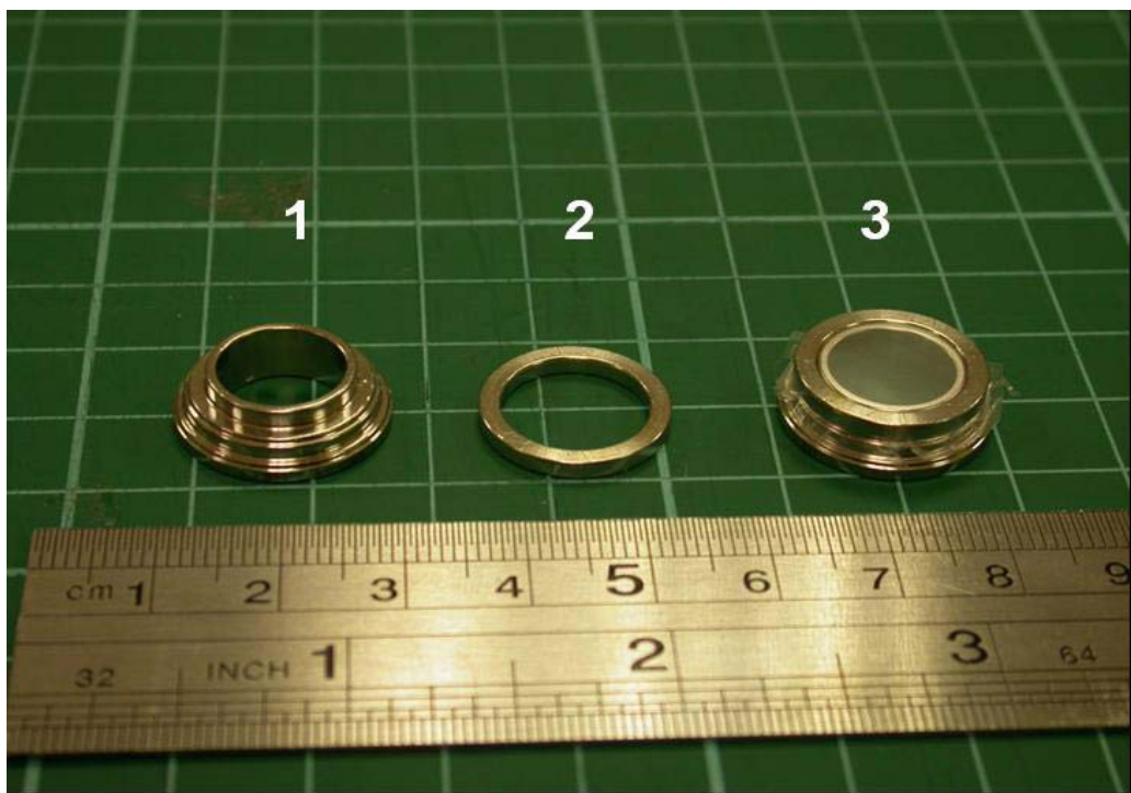
Figure 3-4 Cell-culture-ring. 1 Bottom Part 2.Top part 3.with PCL membrane mounted
