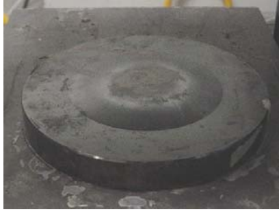
Figure 3.8: Curved strike surface (toughened steel)
