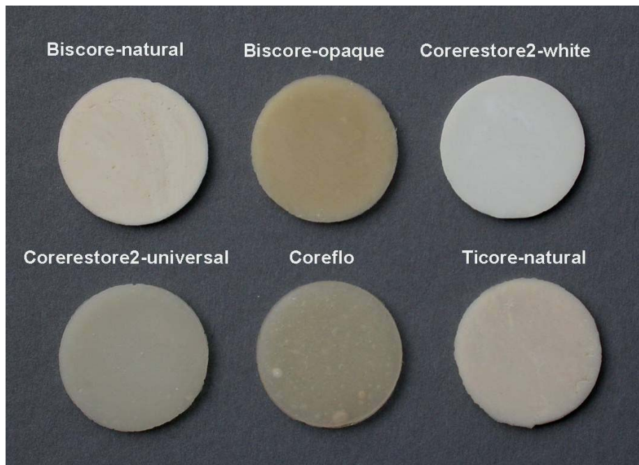
Figure 5b: Specimen disks of composite core materials
