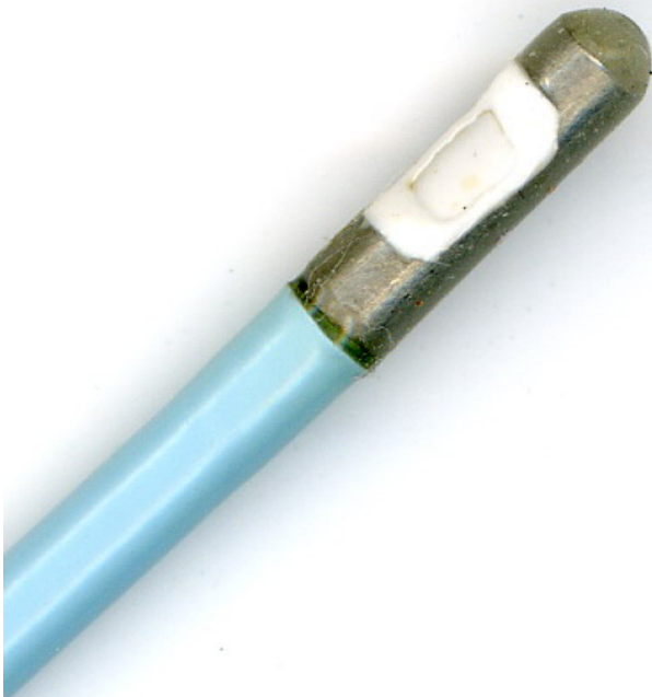
Figure 3.2: The recessed sensing area of the Gaeltec® transducer tip
