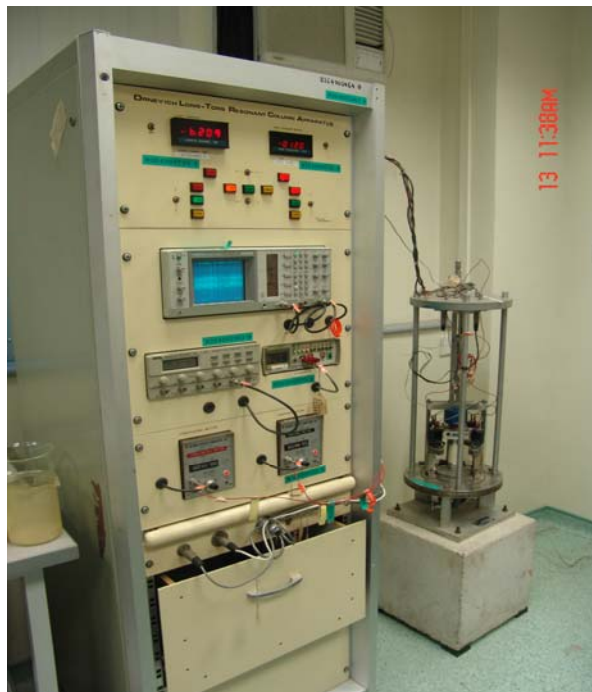
Figure 3.8 Hardin-Drnevich resonant column apparatus
