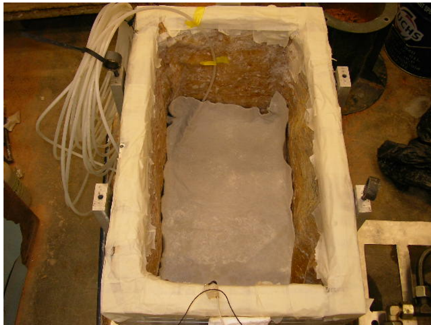
Figure 4.3 Laminar box without soil
