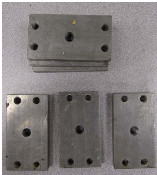
Figure 5.2 Steel plates to simulate added masses
