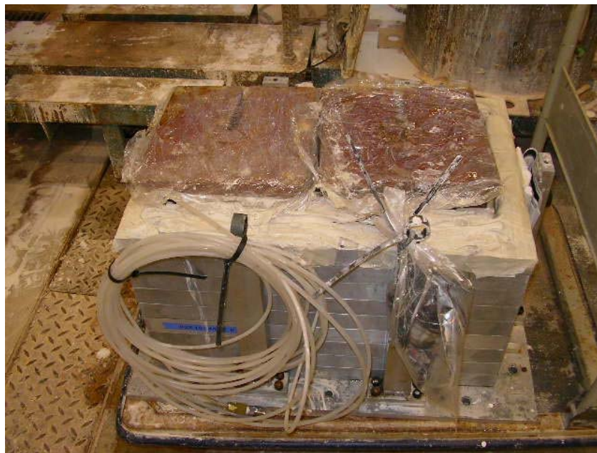
Figure 4.9 1-g consolidation of clay model under dead weights
