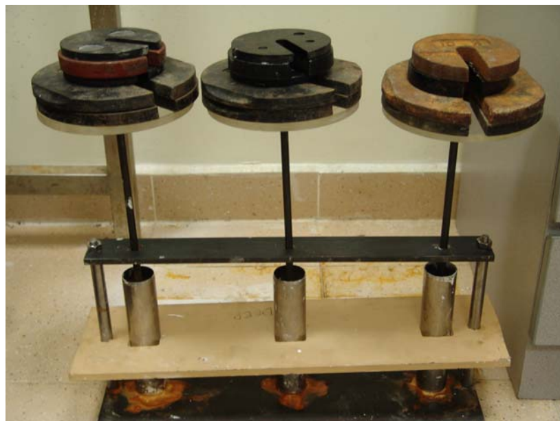
Figure 3.2 Preparation of kaolin clay specimens
