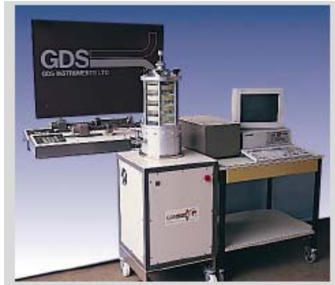
Figure 3.3 GDS advanced triaxial apparatus
