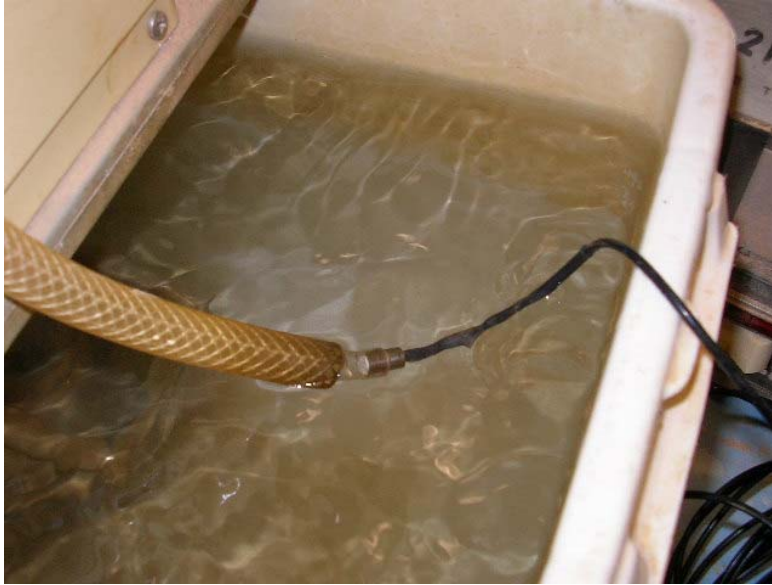
Figure 4.7 Saturation of pore pressure transducer (PPT)
