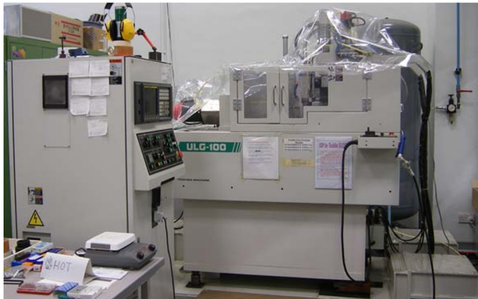
Figure 2.4: A photograph of the entire diamond machining lathe. On the left is the computer system where the programming codes are entered while on the right is the part of the machine which handles the cutting. That part is covered with plastic sheets and doors for safety reasons.
