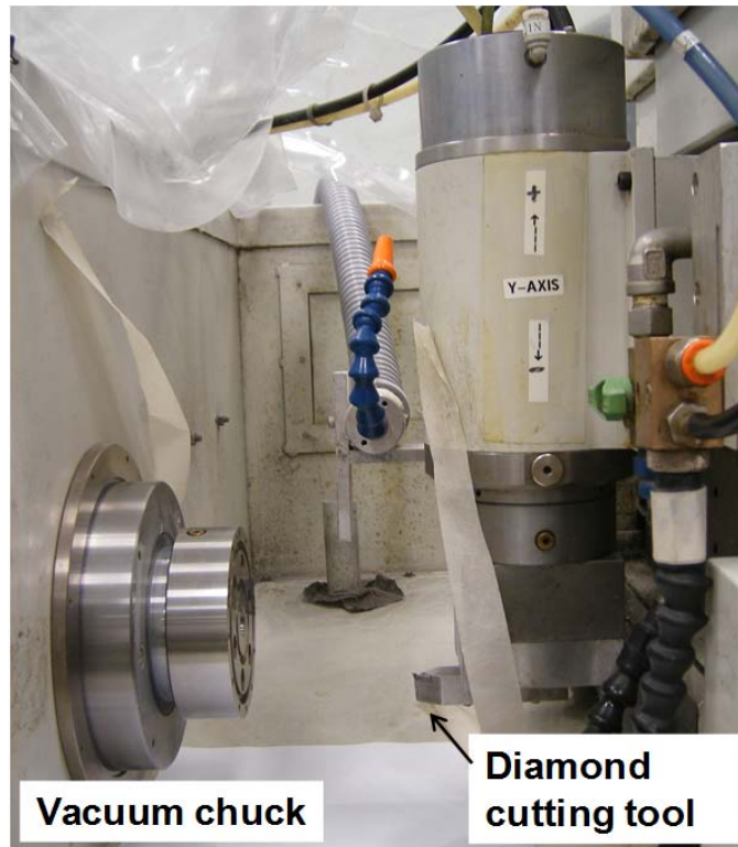
Figure 2.5: A photograph shows the vacuum chuck and the diamond cutting tool on the lathe while not in operation.
