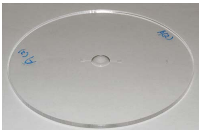
Figure 2.14: A photograph of a diamond turned lens and two shaped liquid channels on a piece of clear PMMA plate.
