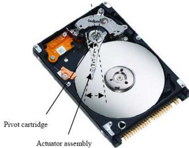
Figure 4.1: Overview of HDD with actuator assembly (source: [4])
