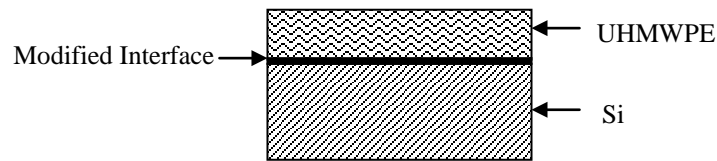
Figure 6.1: A schematic diagram of the Si/UHMWPE sample with different interfaces. Interfacial conditions used were bare Si (i.e. no interface modification), heated Si, APTMS, hydrogen-terminated Si and OTS.
