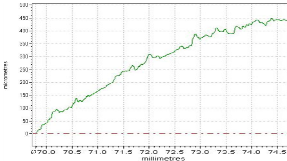
Figure 7.7: Profile of pre-dressed #1200 wheel surface measured with touch probe after scrapping off the oxide layer
