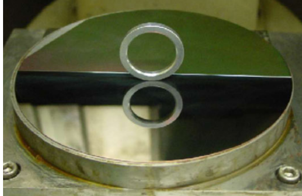
Figure 2.10: Mirror surface generation on Si wafer [30]
