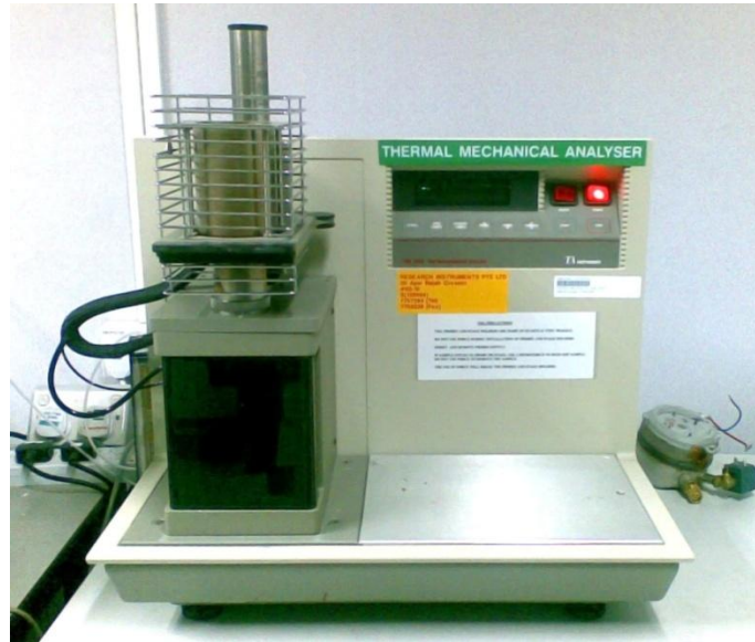
Figure 3.19: Photo of TA instruments TMA 2940, the TMA used in this study
