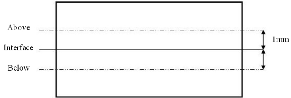
Figure 4.29: Location of areas subject to composition and Vickers hardness testing.
