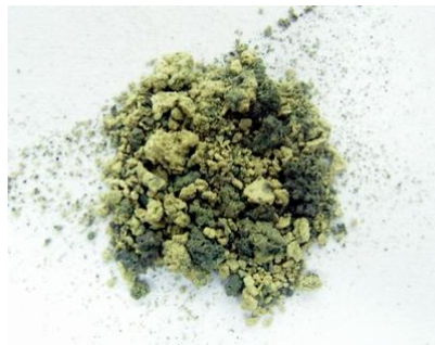
Figure 4.18: Tungsten trioxide ( \text{WO}_3 ) extracted from the sides of the crucible after microwave sintering.
