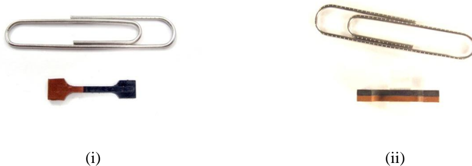
Figure 3.6: Photos showing overmoulded tensile bars, (i) Micro tensile bar with two halves made from copper and tungsten, (ii) Micro tensile dual layer bimetallic bar made from copper and tungsten.
