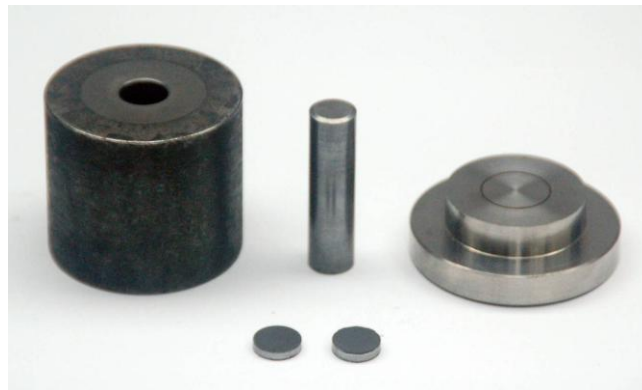
Figure 3.11: Photo showing components of the PM process clockwise from left, the punch, the die, the base and two pressed tungsten discs.
