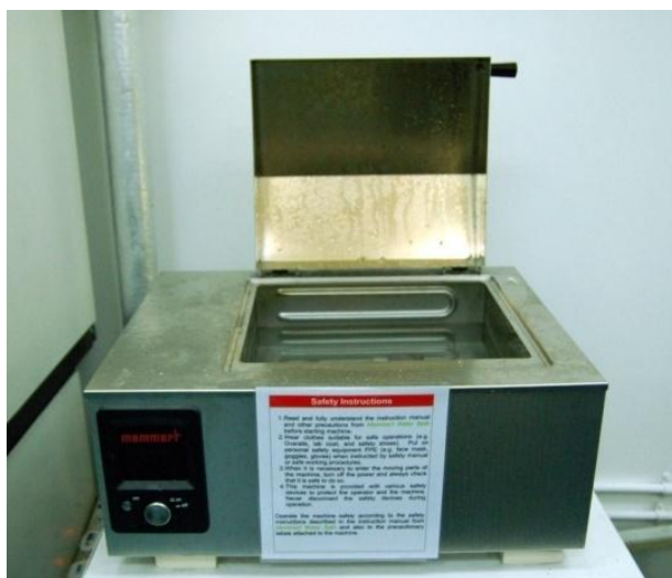
Figure 3.8: The Memmert WNB 45 waterbath used in the solvent debinding process.
