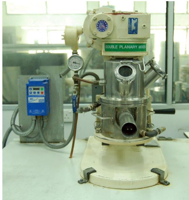
Figure 3.4: Photo of the Ross planetary mixer used in the mixing process
