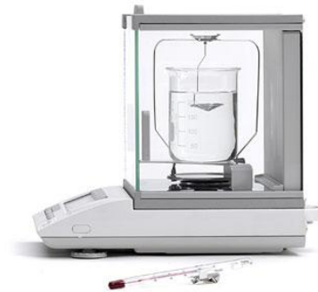
Figure 3.20: Density Determination kit. (Top cone is for measuring w_{air} lower cone is for measuring w_{water} )
