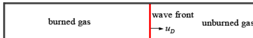
Figure 1.5 ZND detonation propagation in a tube closed at one end
