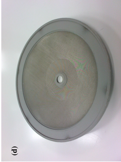
Fig.11. Photographs of the (a) 2 % open area plate, (b) 6 % open area plate, (c) Feidler plate and (d) Tressen mesh of the Wurster coater.
