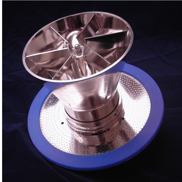
Fig. 12. Photograph of the air distribution plate of the Precision coater attached to the swirl accelerator, which is inverted to show the swirl vanes.
