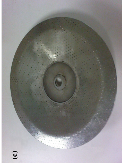
Fig.11. Photographs of the (a) 2 % open area plate, (b) 6 % open area plate, (c) Feidler plate and (d) Tressen mesh of the Wurster coater.
