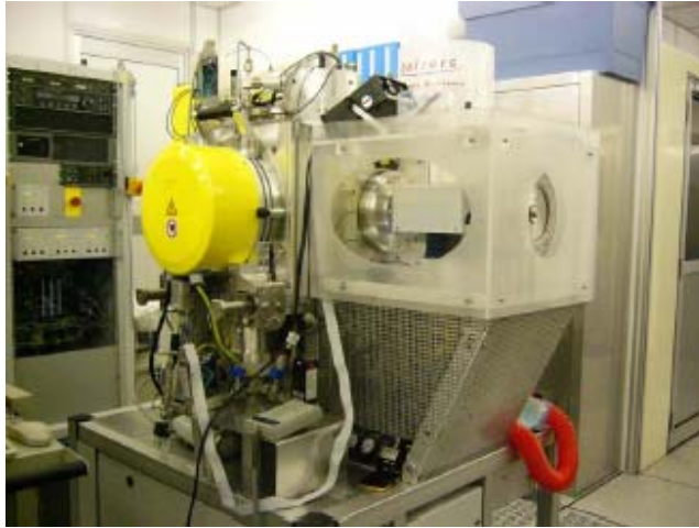
Fig. 6. 6 Balzers sputtering machine used to deposit phase change, dielectric and metal thin films.
