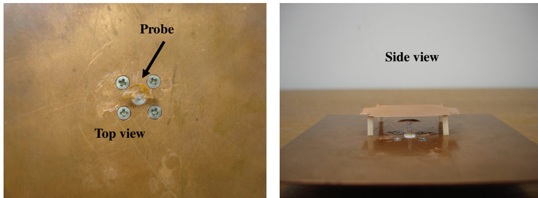
Fig.4.10: Photographs of the fabricated semi-circle probe-fed stub patch antenna.
