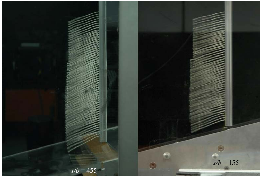
Figure 3.27. Tuft visualization for adverse pressure gradient case with blowing, Re_j = 2660 .
