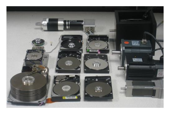
Figure 5.31 Photo of PMSMs tested with integrated drive.
