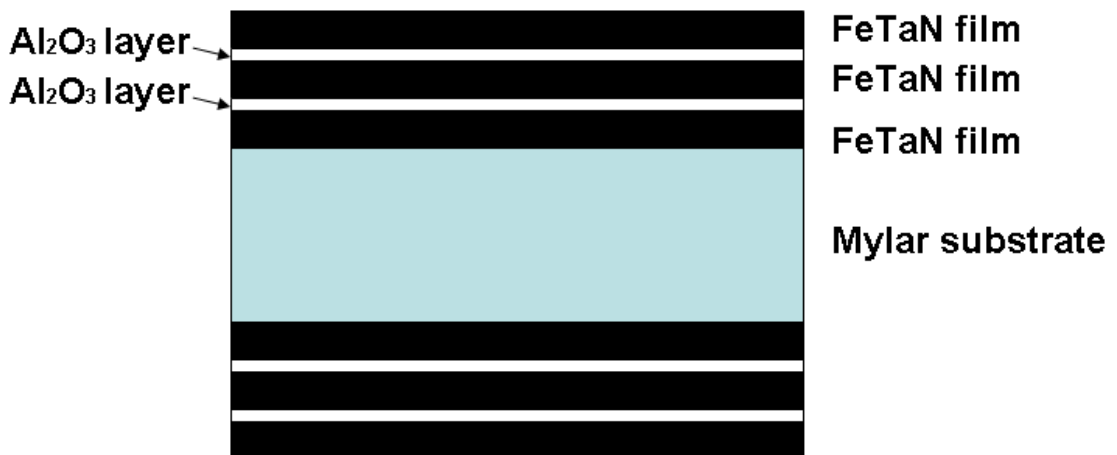
Figure 4.1 Structure of one unit of FeTaN lamination stack
