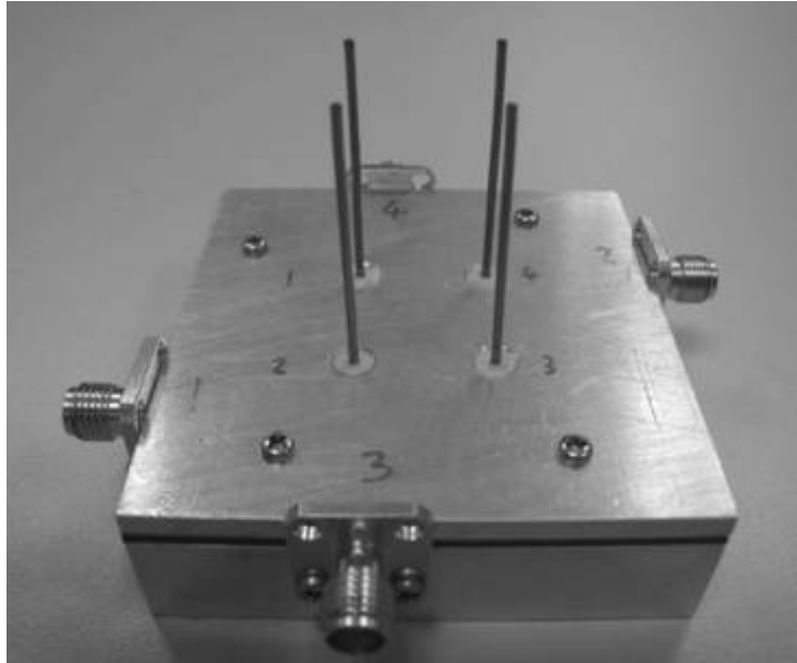
Figure 5.23 Prototype 2 \times 2 element monopole array with decoupled ports
