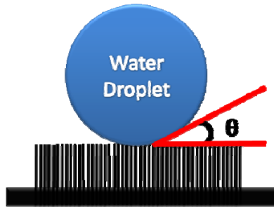
Figure 2.3 Schematic diagram of contact angle measurement, \alpha = 180^\circ - \theta by drawing two tangential lines between the droplet and MWNTs samples.
