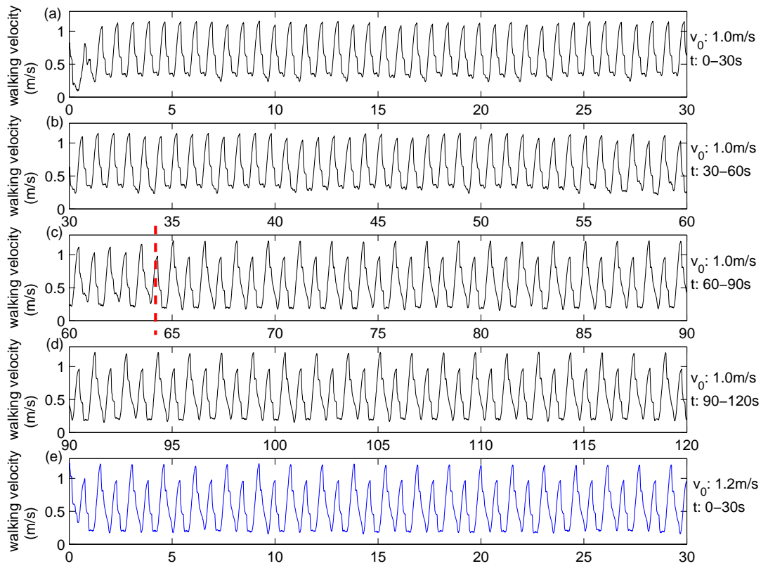
Figure 4.20: Walking velocity profile of motions with further bigger velocity asymmetry under different initial walking velocity v_0 .
