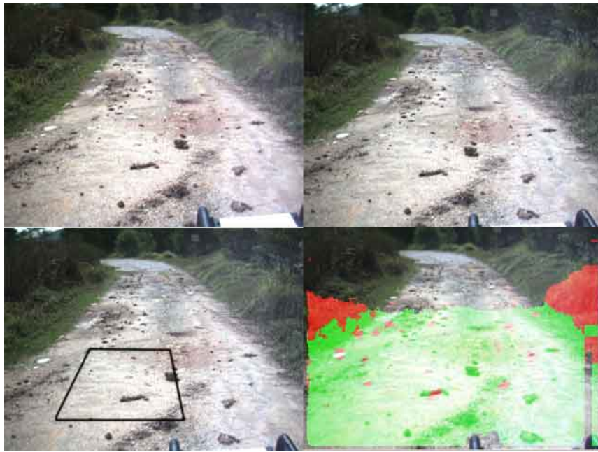
Figure 4.1: Learning region (black trapezoid) and detected ground plane (tinted green) from a pair of stereo images (top images).
