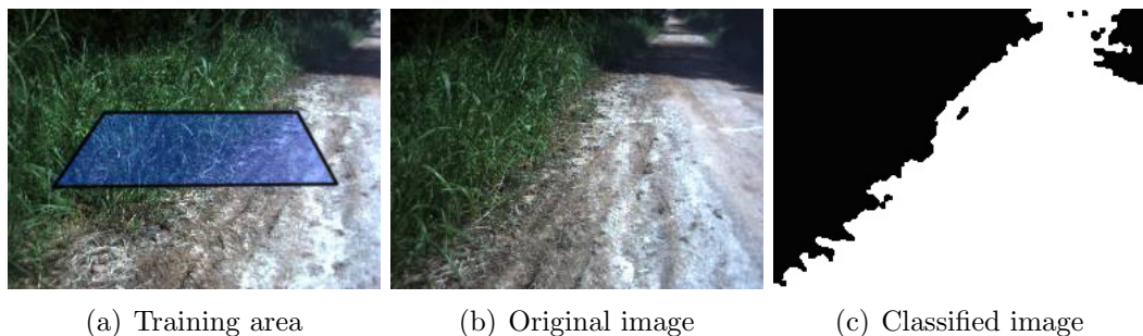
Figure 4.3: Green vegetation removal using look-up table. Grass area does not get trained and model remains valid.
