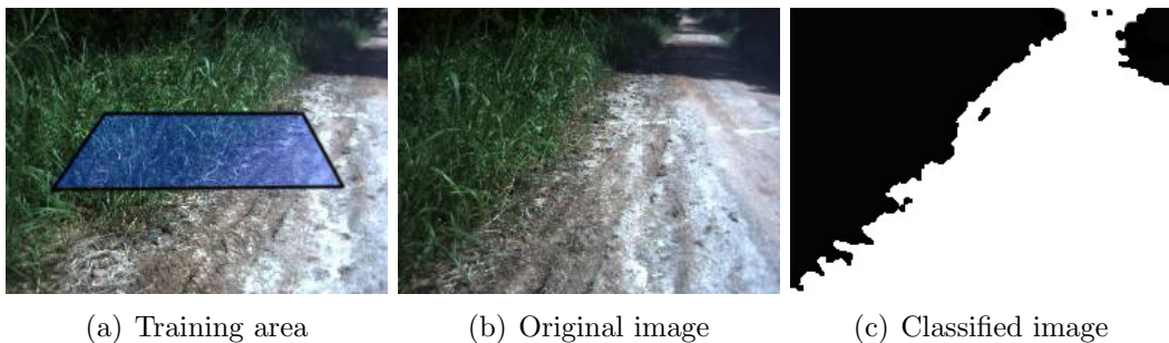
Figure 4.4: Green vegetation removal using pre-trained Gaussian mixture. Grass area does not get trained and model remains valid.
