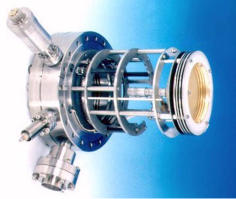
Figure 2.1. Above: Schematic set-up of a LEED experiment. Below: a LEED optics assembly produced by Omicron (picture courtesy of Omicron).
