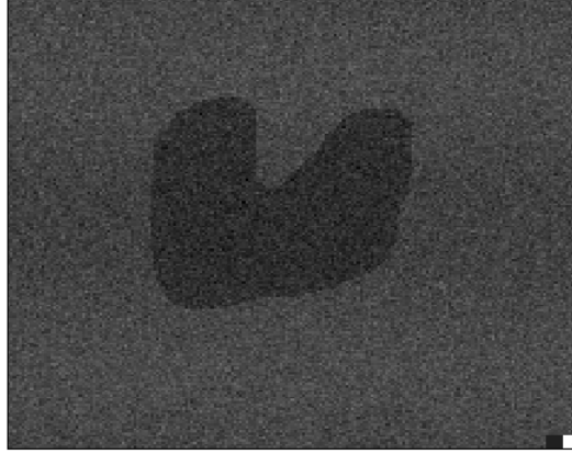
Figure 4.6: Computer generated image corrupted by noise and bias
