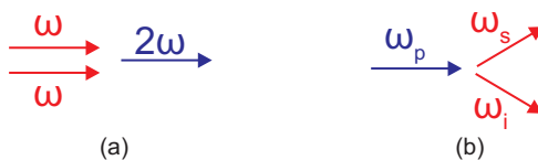
Figure 2.4: Feynman diagrams for second-order nonlinear processes. (a) Second harmonic generation or frequency doubling. Two pump photons of the same frequency \omega get annihilated producing an output photon of frequency 2\omega . (b) Down-conversion. A pump photon of frequency \omega_p gets annihilated producing two photons at the signal and idler frequencies \omega_s and \omega_i , respectively. The sum of the signal and idler frequencies \omega_s and \omega_i is equal to the pump photon frequency \omega_p .
