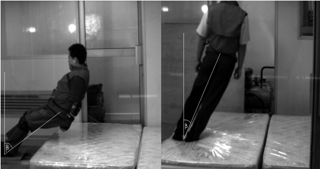
Figure 5.14. Typical body configuration at threshold level for backward fall and sideways fall.
