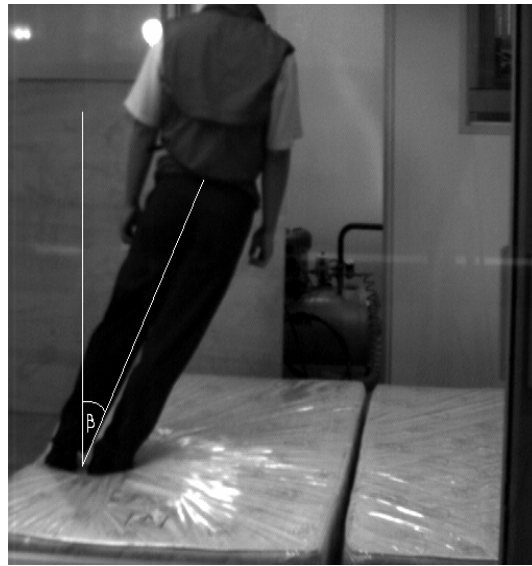
Figure 5.7. Angle of body configuration at the threshold level
